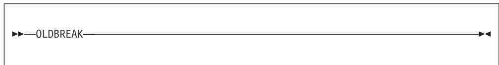
The OLDBREAK option sets an alternative mode of operation for the BREAK command. This mode of operation does not "toggle" a breakpoint. If the BREAK command is issued against an address where a breakpoint is already set, IDF issues an error message.
