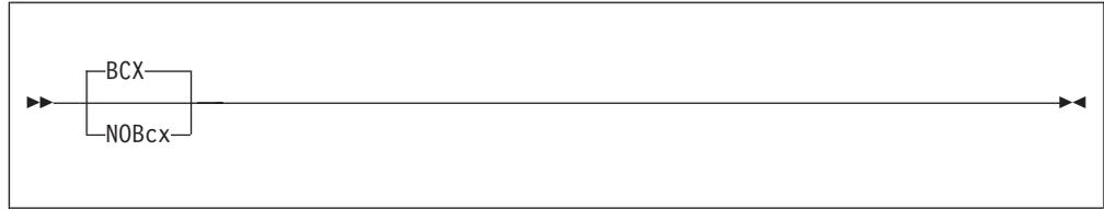
When the instruction displayed on the main panel is a BC or BCR, BCX shows an extended branch mnemonic instead of the CC mask when disassembling the instruction. Mnemonics used are those for use after compare instructions. This option has no effect on branch relative instructions.
