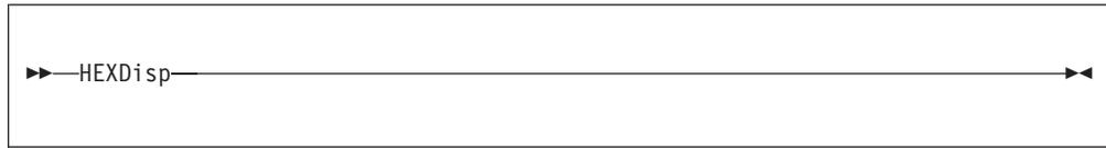
When the HEXDISP option is set, hexadecimal notation is used in disassembled instructions for all displacements from symbols, or displacements which cannot be related to symbols.
