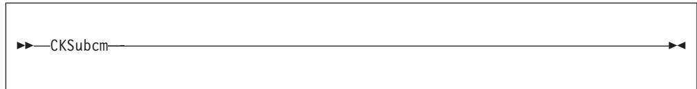
When the CKSUBCM option is set, IDF checks that its subcommand environment is intact before executing a REXX exit routine. The CKSUBCM option is intended for use in hostile environments which cut off the subcommand chain.
