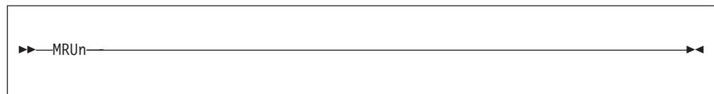
The MRUN command is different to RUN, because the target program is executed *before* control returns to the issuing macro. When RUN is issued from a macro, it has no immediate effect, being processed *after* the macro exits.
