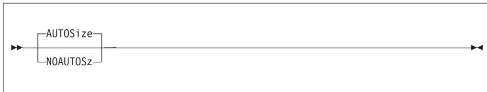
AUTOSIZE tells IDF to automatically size Disassembly windows, Dump windows, and LSM Information windows when a window is opened or closed. IDF also automatically places all opened windows so that each window's upper border overlays the lower border of the window last opened.
