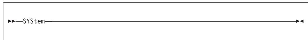
When the SYSTEM option is set, the program runs in system key (key=0).
