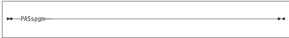
The PASSPGM option makes IDF pass program interruptions that are not the result of a PER event to the CMS, z/OS or z/VSE program interrupt handler. Used for debugging exit routines.
