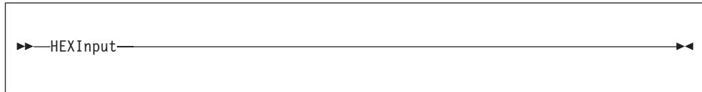
When the HEXINPUT option is set, IDF assumes that numbers input without any explicit indication of base are hexadecimal. If the first digit of a hexadecimal constant is not zero, IDF interprets it as the name of a symbol.
